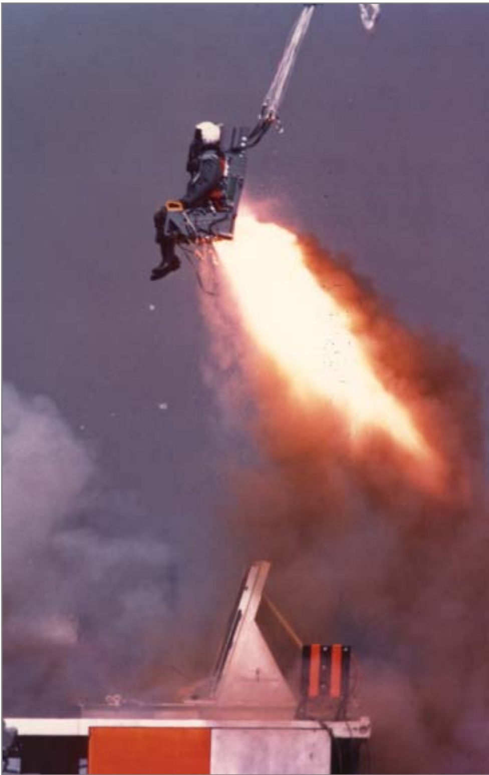
Testing of advanced pilot ejection seat
