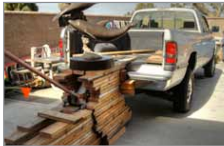
Maintenance at work on the lifting mechanism. Floor jack and lumber brings statue to truck bed height.
