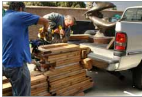
Maintenance at work on the lifting mechanism. Floor jack and lumber brings statue to truck bed height.
